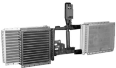
Figure 24. Air-to-air, fixed-plate heat exchanger recovers sensible energy
