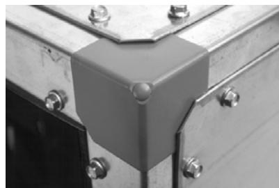
The flush-mounted access doors with integral thresholds (see Figure 8) limit the seams in the unit casing, which reduces locations for dirt to collect. The integral door threshold and heavy-duty door fit together to assure a tight seal for the life of the air handler.
