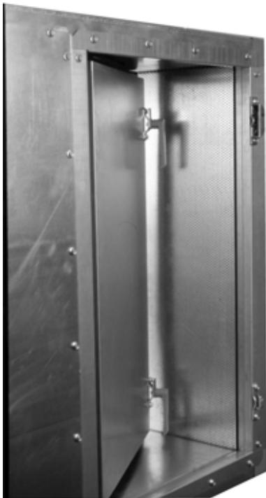
Heavy-duty door handles and hinges are surface-mounted, eliminating a potential leakage path since they do not pierce the casing. A removable hinge pin allows for easy door removal; the symmetrical handle and hinge mounting allows for easy field modification if it becomes necessary to change from a left-hand to a right-hand door.
