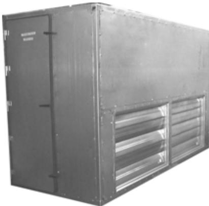
A mixing box module typically combines the incoming outdoor air with recirculated return air collected from the occupied space. It is commonly included in an air handler design to control this mixture. When equipped with an optional Traq damper, the mixing box module permits direct measurement of outdoor airflow to assure compliance with ASHRAE Standard 62.1.
