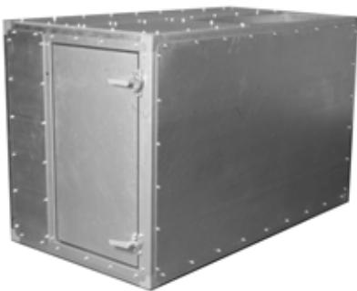
Before leaving the air handler, supply air can be ducted to a discharge plenum module. The rapid air-stream expansion as it passes into the plenum reduces turbulence and creates an acoustical end reflection that dampens low-frequency sound. Two configurations enable supply-duct connections from any side:
