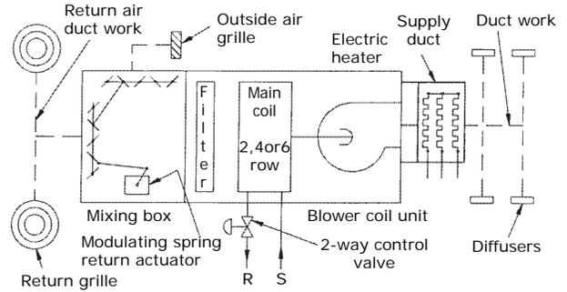
**Figure 8. Two-pipe with changeover typical application**
