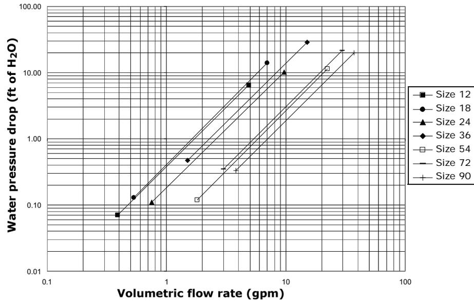
Figure 20. Six-row high-capacity cooling coil water pressure drop
