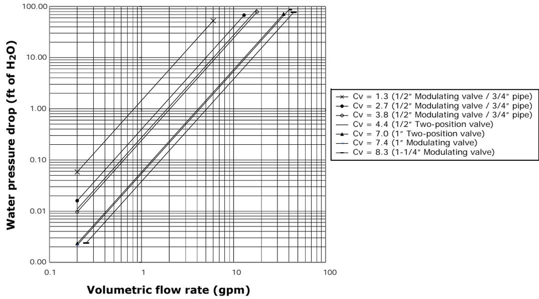
Figure 16. Three-way deluxe piping package water pressure drop
