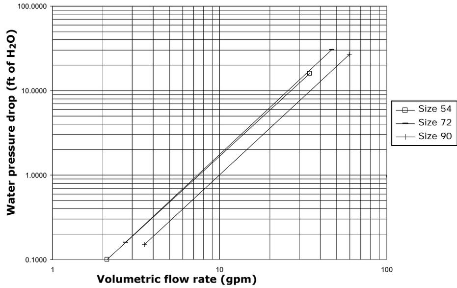
**Figure 18. Six-row standard cooling coil water pressure drop**
