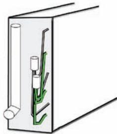
**Figure 12. Horizontal face split DX coil**
