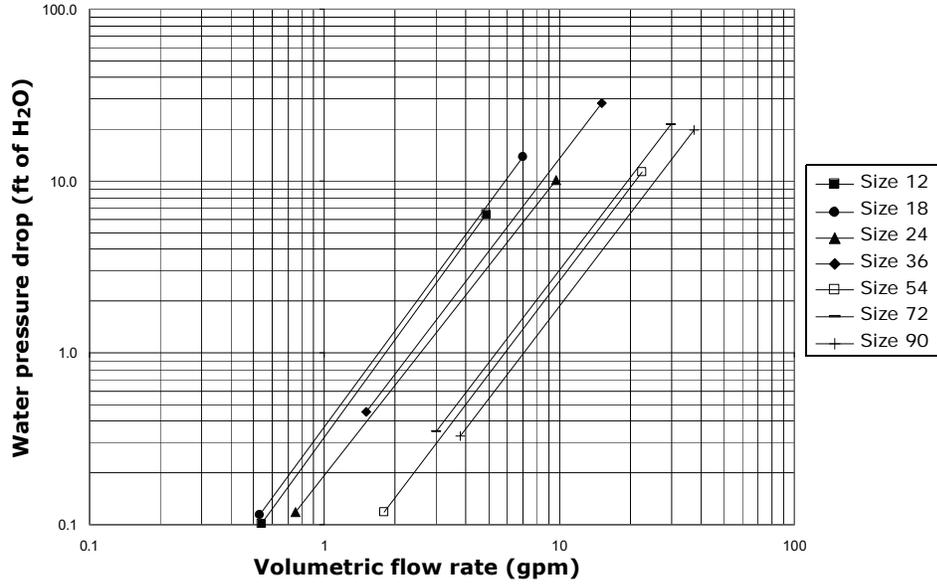
Figure 26. Six-row high-capacity heating coil water pressure drop
