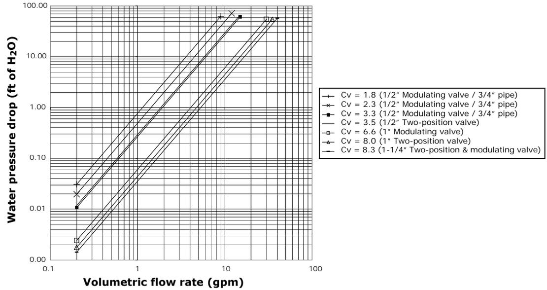
Figure 14. Two-way deluxe piping package water pressure drop
