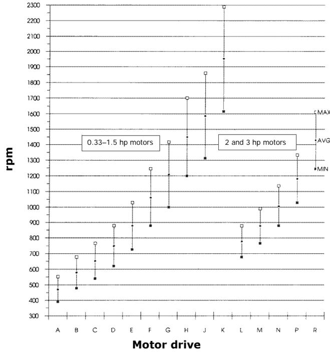
Figure 47. Size 12-90 drives, 50 Hz motors
