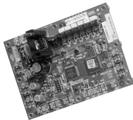
**Figure 39. Tracer ZN520 control board**
