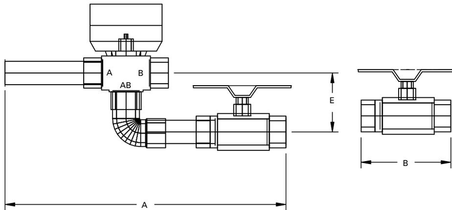
**Three-way, 1/2" and 1" valve basic piping package**
