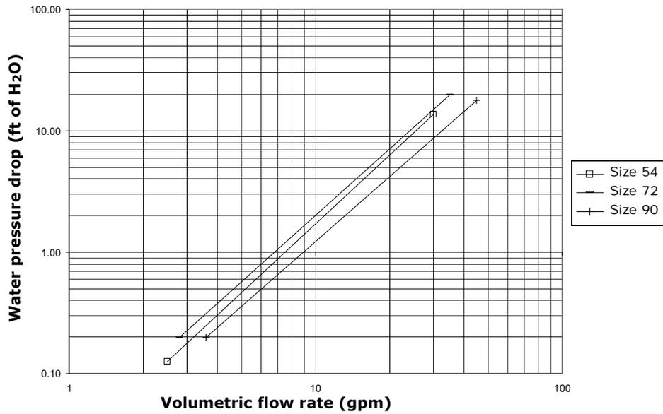
Figure 24. Two-row high-capacity heating coil water pressure drop
