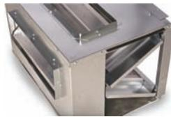
Filter box options include an angle filter box and a bottom/top access filter box that are factory-installed. The angle filter can be combined with the mixing box as one accessory module. The flat filter frame can accommodate 1- or 2-inch filters. The angle filter frame accommodates only 2-inch filters. See [Figure 4](#).
