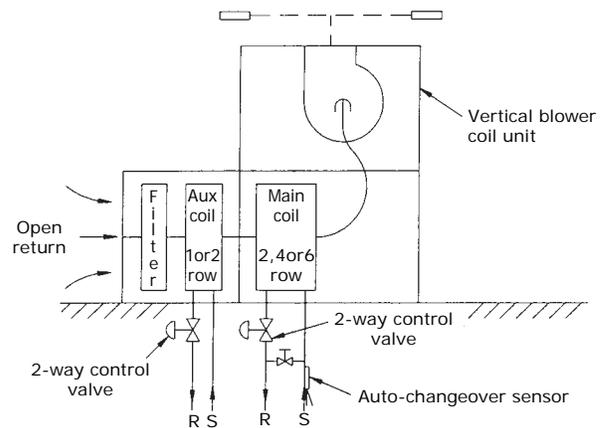
**Figure 10. DX with hot water preheat typical application**
