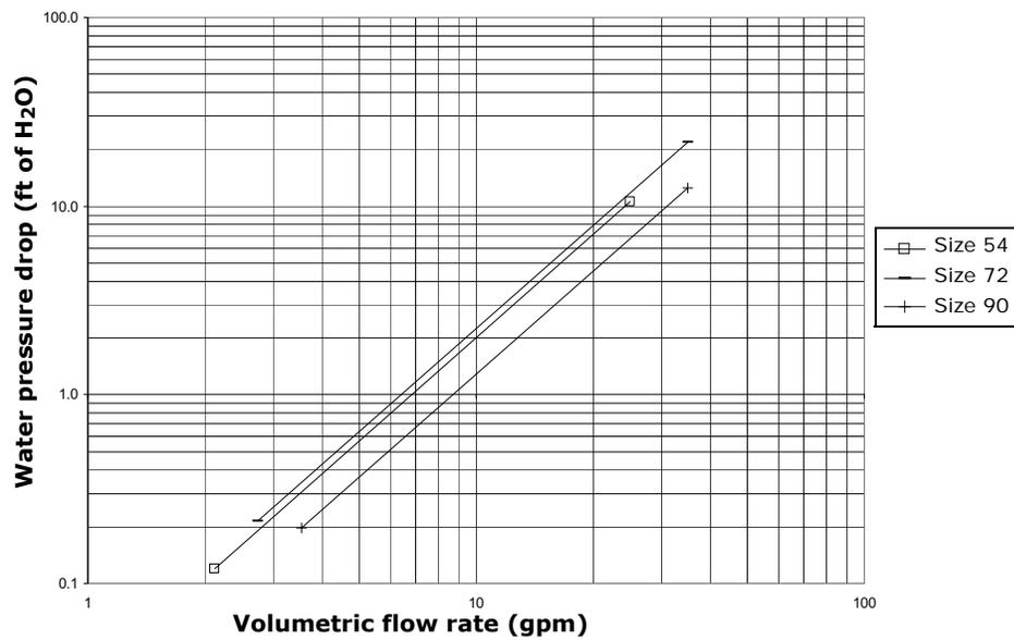
Figure 19. Four-row high-capacity cooling coil water pressure drop
