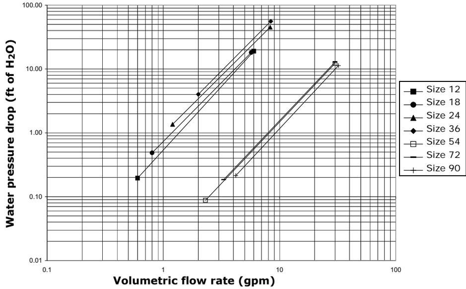
**Figure 22. Four-row standard heating coil water pressure drop**
