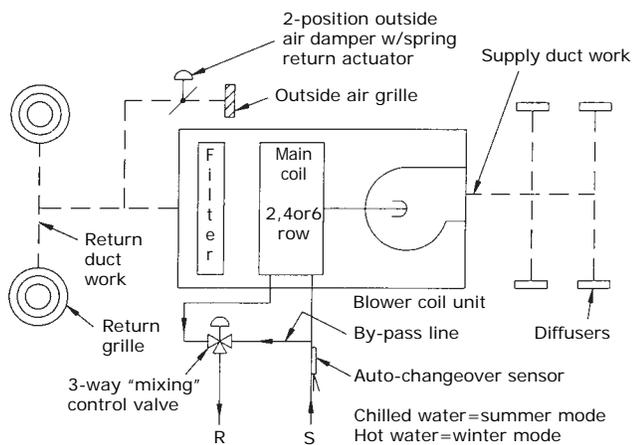
**Figure 9. Four-pipe vertical with changeover typical application**
