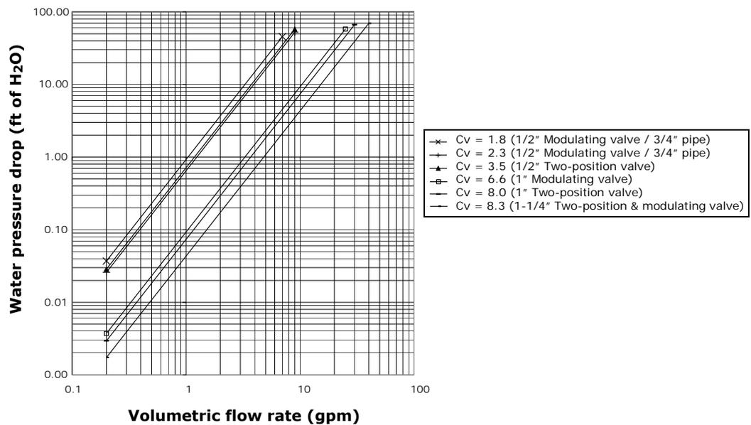
Figure 15. Three-way basic piping package water pressure drop
