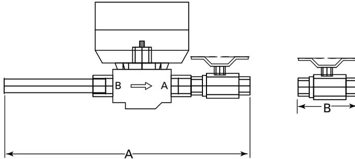
**Two-way, 1-1/4" valve basic piping package**
