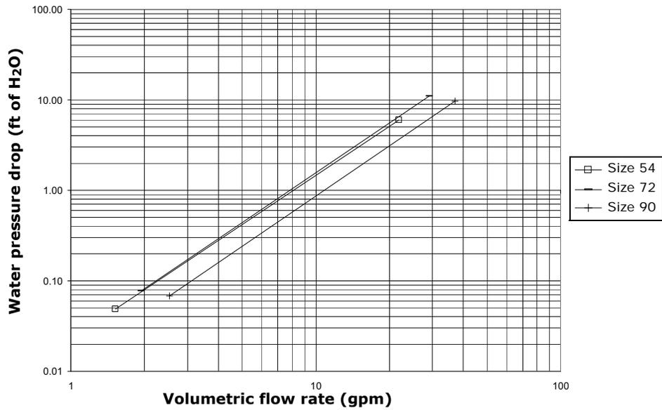
Figure 23. Six-row standard heating coil water pressure drop
